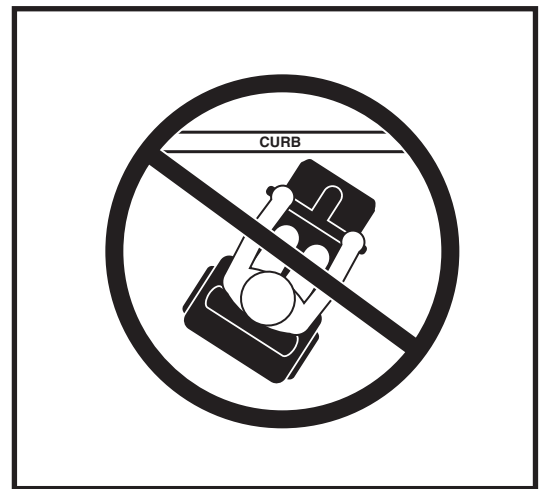
Figure 7. Incorrect Curb Approach
