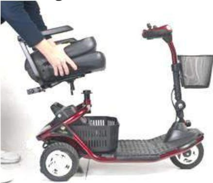
**Figure 13. Removing the Seat**
