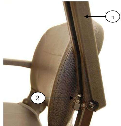
**Figure 7. Flip-up/Angle Adjustment**
