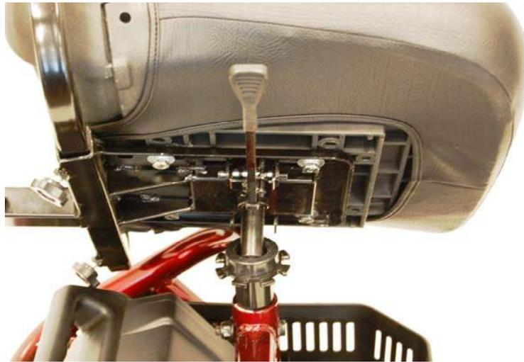
*Figure 23. Installing the Seat*
