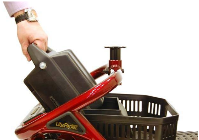
Figure 21. Battery Pack Installation
