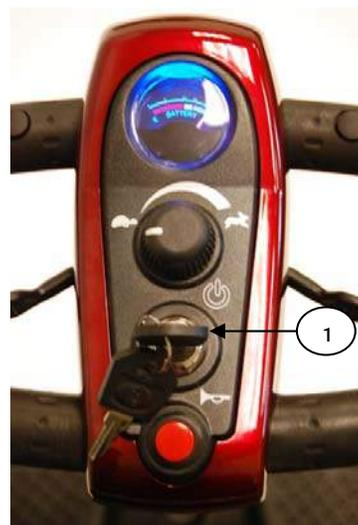
**Figure 12. Key Switch (On)**
