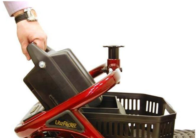
**Figure 21. Battery Pack Installation**
