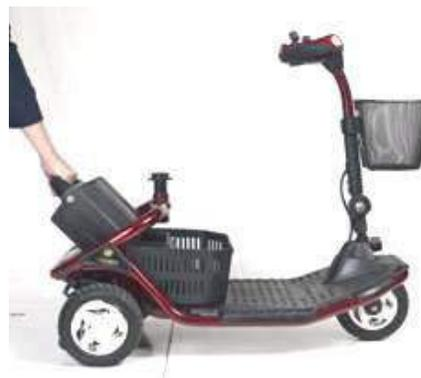
**Figure 14. Removing the Battery Pack**
