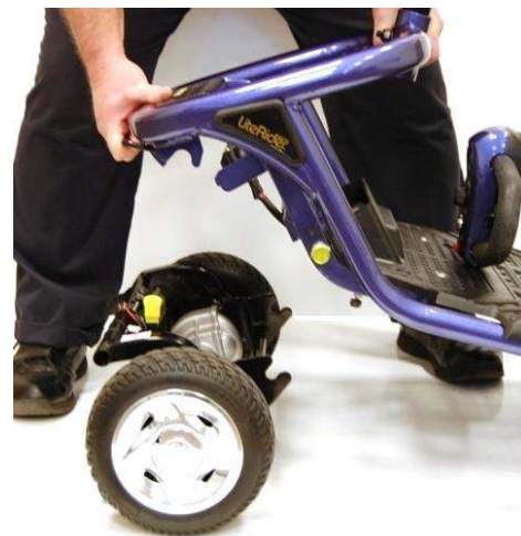
Figure 18. Lifting the Frame
