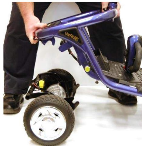
**Figure 18. Lifting the Frame**
