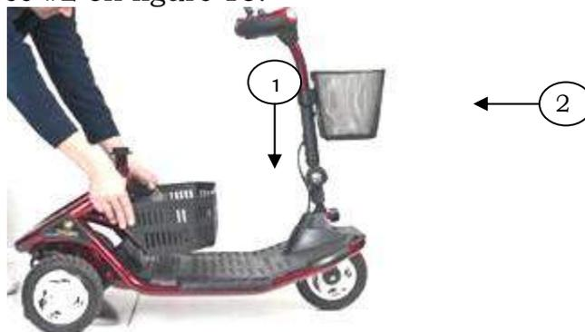
**Figure 15. Removing the Baskets**
