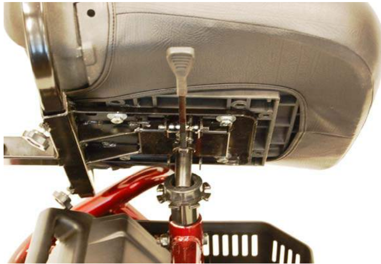
Figure 23. Installing the Seat
