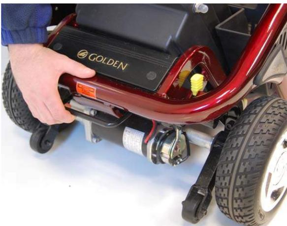
**Figure 17. Releasing the Drivetrain**
