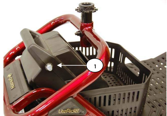
Figure 27. Main Circuit Breaker
